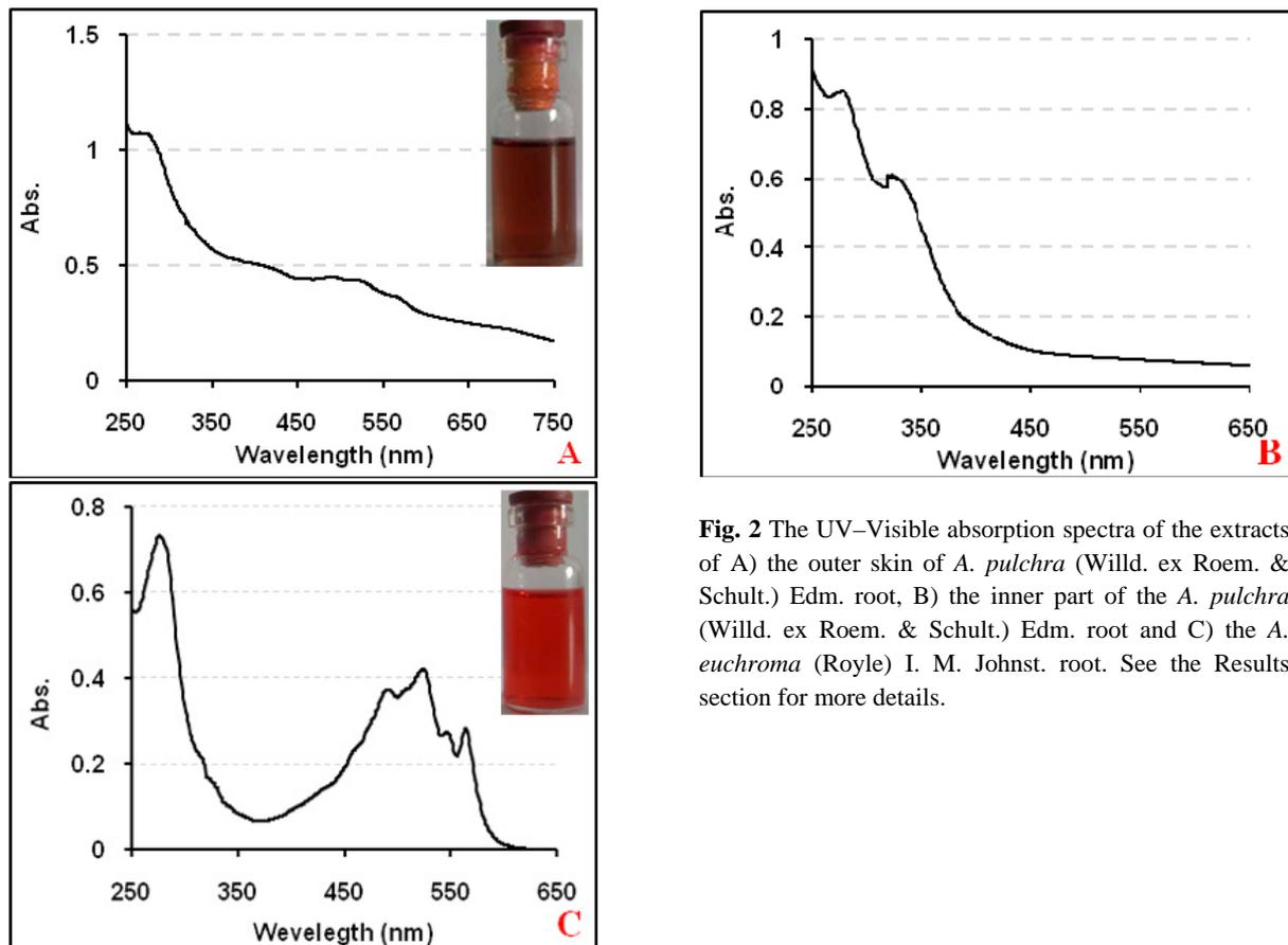
**Fig. 2** The UV-Visible absorption spectra of the extracts of A) the outer skin of *A. pulchra* (Willd. ex Roem. & Schult.) Edm. root, B) the inner part of the *A. pulchra* (Willd. ex Roem. & Schult.) Edm. root and C) the *A. euchroma* (Royle) I. M. Johnst. root. See the Results section for more details.
