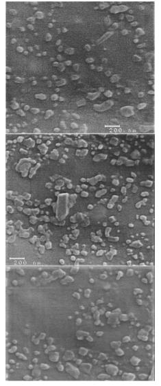
**Figure 2.** Scanning electron microscope micrograph of azelaic acidloaded chitosan, Up: sonicated 120 s (sample No. 18), Middle: sonicated 60 s (sample No. 13) and Down: non-sonicated (sample No. 3).
