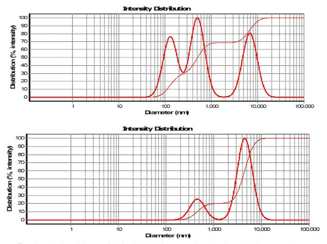
Figure 1. Particle size analysis report of azelaic acid-loaded chitosan, Up: sonicated (sample No. 18, d(50):516 nm) and (B) Down:non-sonicated (sample No. 3, d(50):3990 nm)
