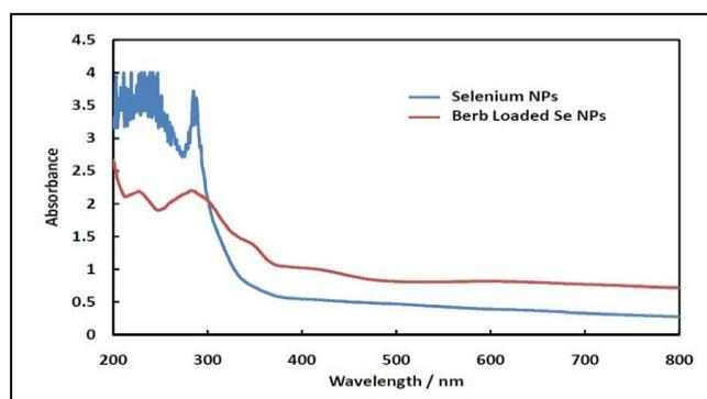
**Figure 1.** The UV- visible spectrum of chemical synthesis of Se nanoparticles upon reduction with ascorbic acid as a reducing agent and vitamin E TPGS as a stabilizing agent
