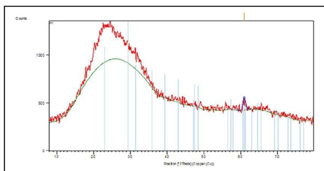
**Figure 2.** X-ray diffraction patterns (XRD) of chemical synthesized selenium nanoparticles (Se NPs) using ascorbic acid as a reducing agent in the presence of vitamin E TPGS as a surfactant
