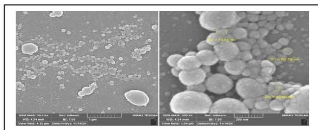
**Figure 3.** Scanning Electron Microscope images of selenium nanoparticles (Se NPs) synthesized by chemical reduction of sodium selenite with ascorbic acid using vitamin E TPGS as a surfactant
