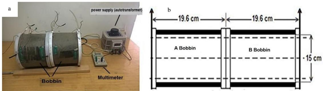
**Fig. 1** Electromagnetic Field Generator. A solenoid generating an extremely low-frequency electromagnetic field (ELF-EMF): a) the internal diameter of each solenoid is 15 cm; b) the effective length is 15.6 cm; the number of turns in solenoid A ( $N_A$ ) is 1756 and in solenoid B is 1732 [25].
